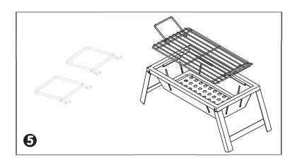
To move the grill while hot, insert the prongs of the handles into the holes in either end of the grill. Lift carefully.
