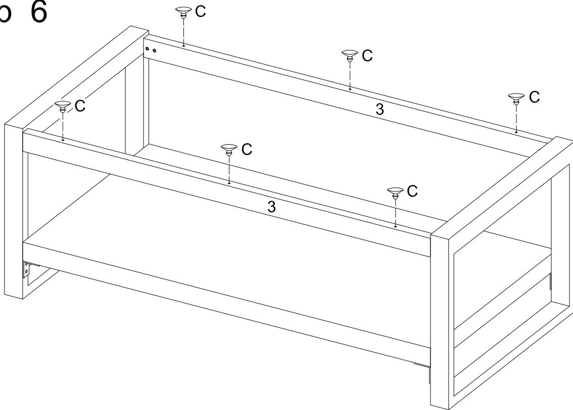
Insert the rubber suction cup into the metal bars (3).
