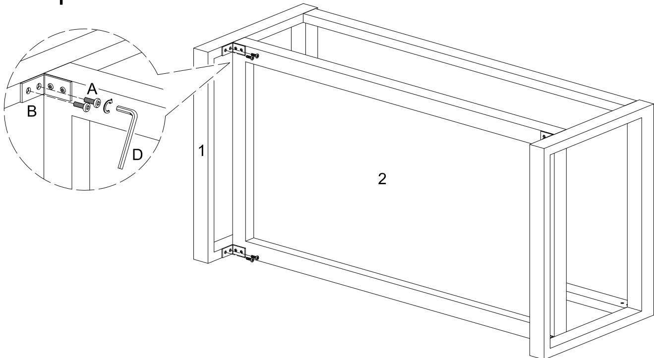
Use bolts (A), wrench (D) to secure the L shape bracket (B) to the side frame (1).
