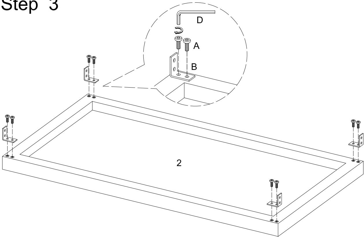
Use bolts (A), wrench (D) to secure the L bracket (B) to the bottom panel (2).
