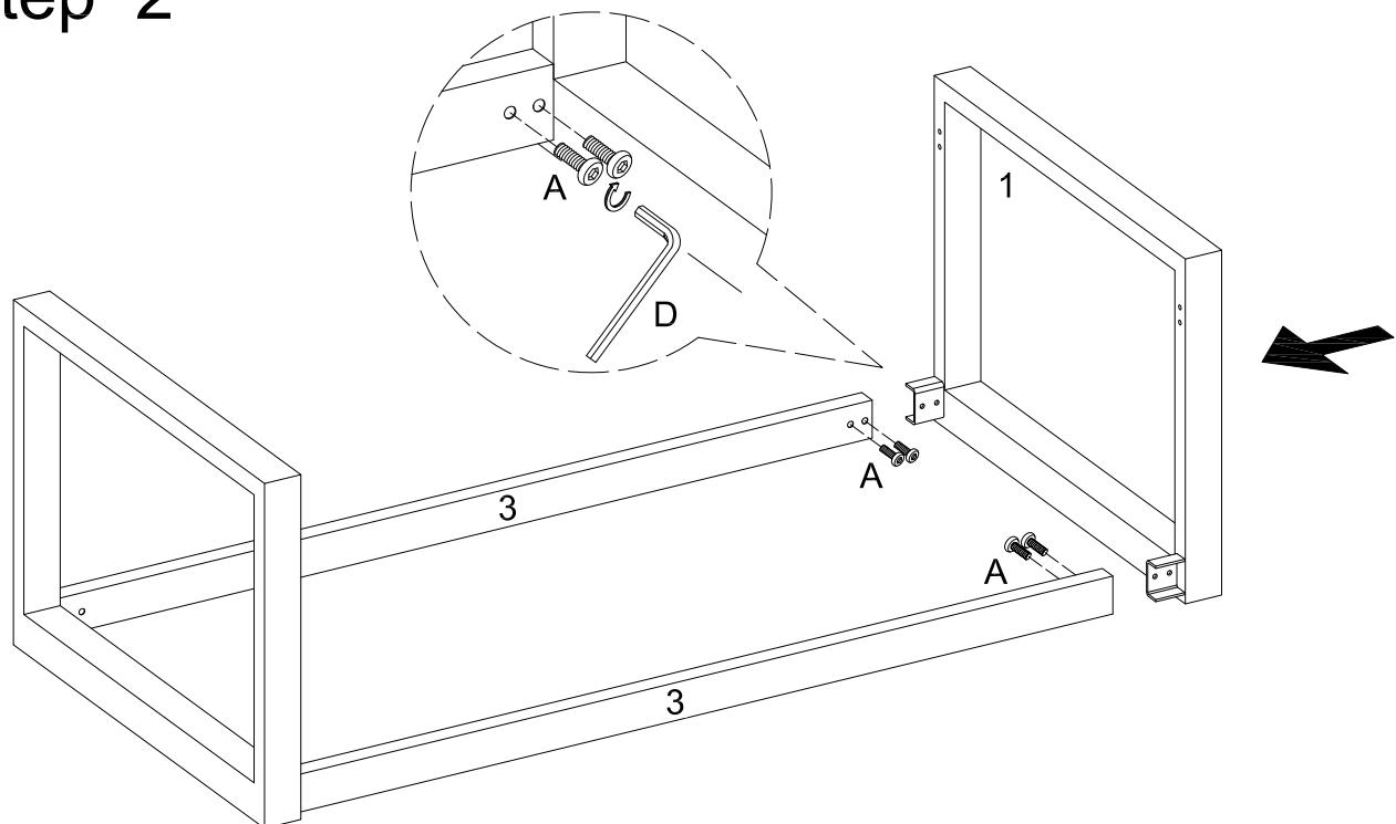
Use bolts (A), wrench (D) to secure the metal bars (3) to the other side frame (1).
