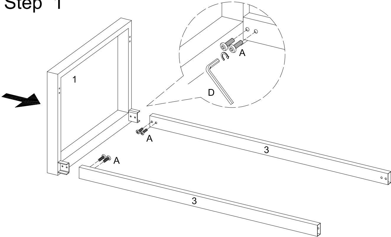
Use bolts (A), wrench (D) to secure the metal bars (3) to the side frame (1).
