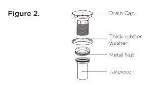
**Step 3:** From under the drain, insert the thick rubber washer, screw on and tighten the metal nut. Romove excess plumbers' putty.
