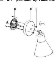
Carefully pass the wires through the moungting plate assembly(B)
