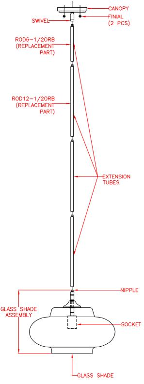
AVAILABLE PARTS ARE: ROD6-1/20RB (6" EXTENSION TUBE) ROD12-1/20RB (12" EXTENSION TUBE) MODEL: 93036AMB
