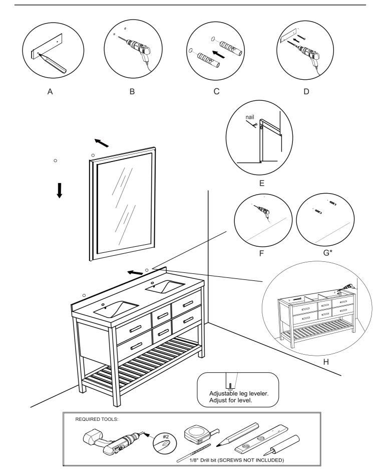
\*SECURE SCREW TO STUDS WHEN POSSIBLE
