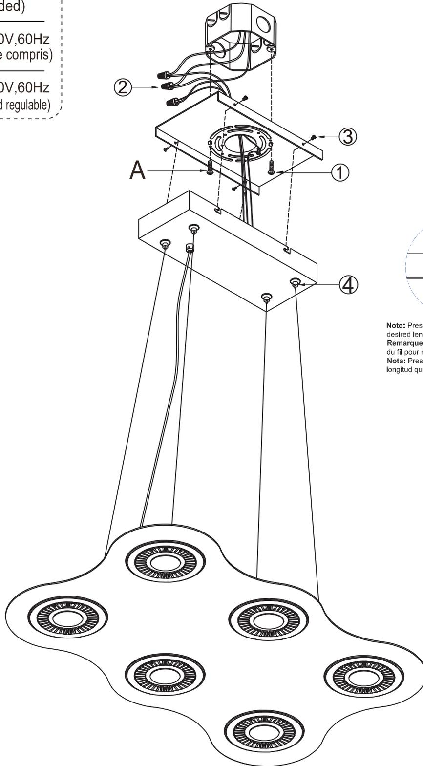
**Note:** Press the wire restraint to adjust the desired length of cable.
