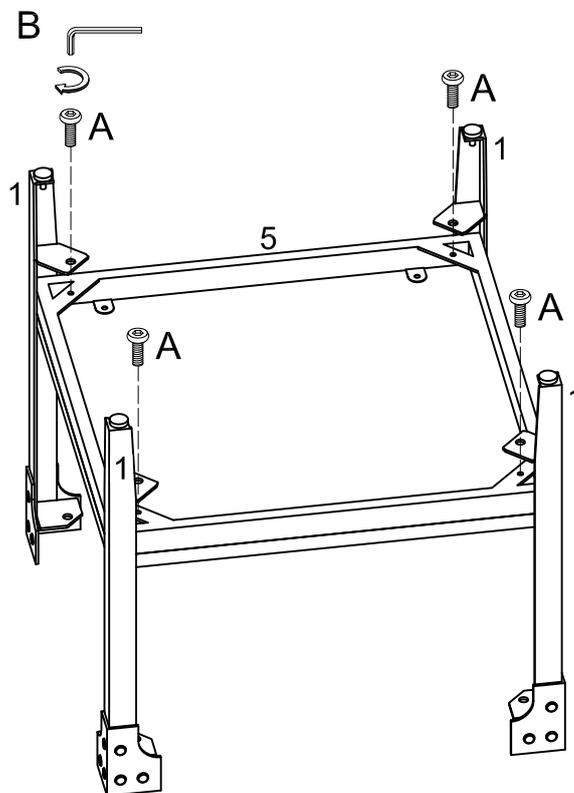
Attach legs (1) to frame (5) using bolts (A) as shown in the diagram.
