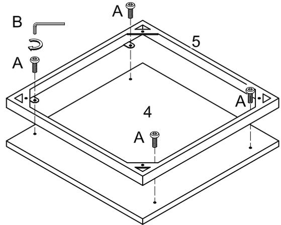
Secure wood panel (2) to frame (3) and wood panel (4) to frame (5) using bolts (A) as shown.
