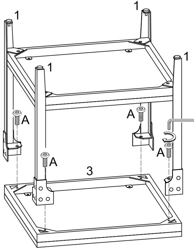
Attach frame (3) to legs (1) using bolts (A) as shown.
