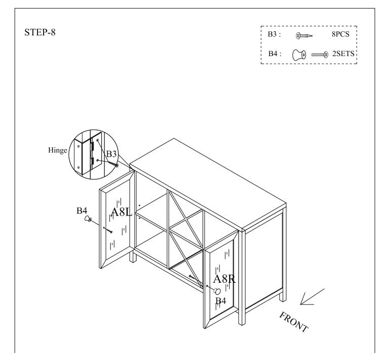
Assemble Doors A8(L&R) with hinges to Side Panels A4(L&R) using Screws B3.
