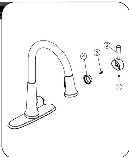
Shut off water supply. Unscrew the set screw (1) on the handle (2). Remove handle (2) and unscrew the screw (3). And then remove cap (4).
