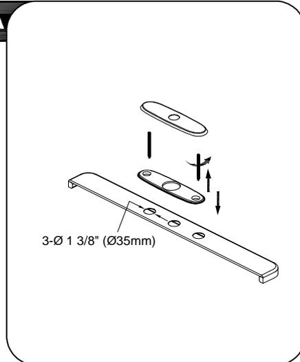
Before installation, screw bolts to the large escutcheon.
