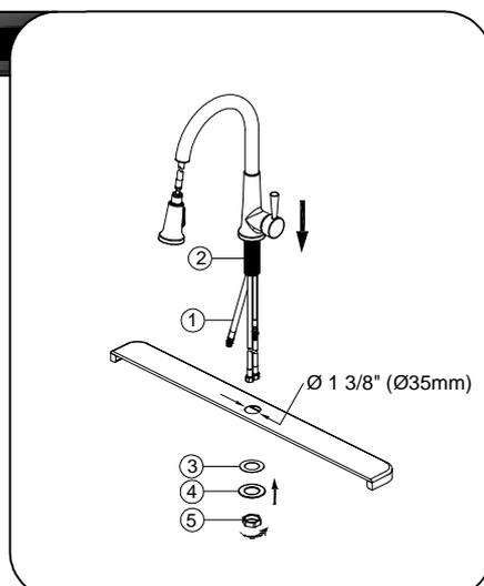
Retract pull-out hose (1) up through faucet body, until the pull-out hose fitting is flush with the bottom of shank (2). Do not pull hose fitting past the shank. Insert faucet body through the hole.
