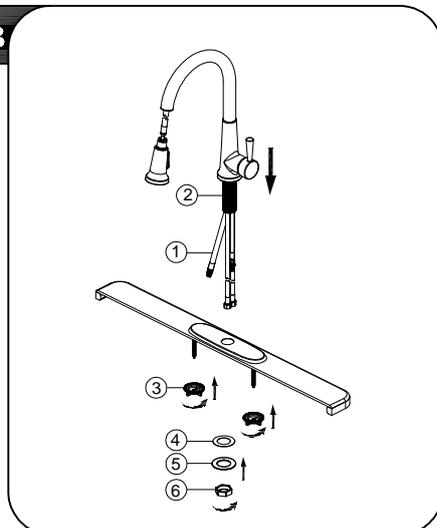
Retract pull-out hose (1) up through faucet body, until the pull-out hose fitting is flush with the bottom of shank (2). Do not pull hose fitting past the shank. Insert faucet body through the hole in escutcheon.
