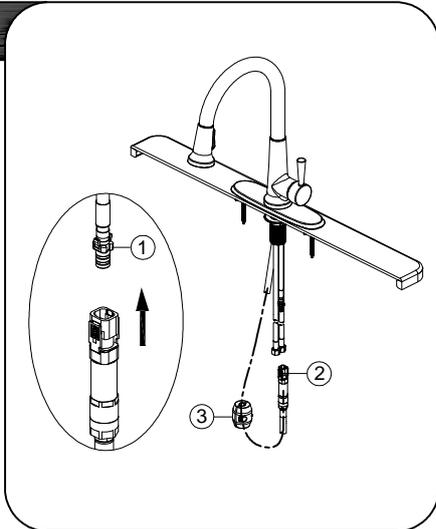
Screw quick connect assembly to the free end of pull-out hose. Align male fitting (1) and tabs (2) on quick connector. Push quick connector housing firmly upward and snap onto receiving male fitting. Pull down moderately to ensure connection has been made.
