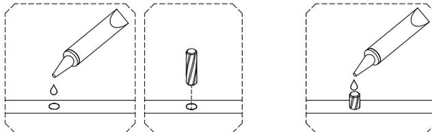
1: The provided glue is to secure wood dowels in place. When first inserting dowels, locate the appropriate hole for the dowel, place a small amount of glue in the hole and insert the dowel. Wipe away excess glue immediately.
