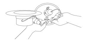
5 Squeeze torsion springs together and install into torsion spring brackets inside recessed housing.
