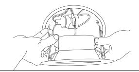
6 Carefully route wires into housing and push the downlight upward, flush to ceiling surface.
