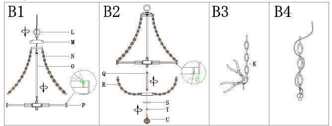
Step B1: Thread the tube (O)onto the threaded nipple on the fixture (P), the upper bead strand assembly (N) and double cover (M) are then fixed on the tube (O) with the ring (L). Carefully hang the bead strands onto the fixture (M).
