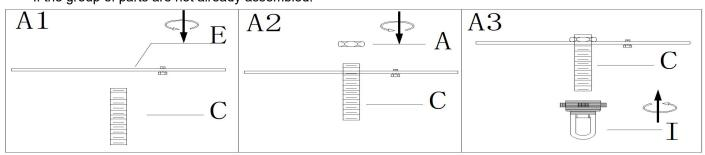
Step A1: Thread the single bar(E) over the nipple (C) a minimum of 6 mm (1/4"). At this point need note that: the side of single bar marked "GND" must face to the down.
