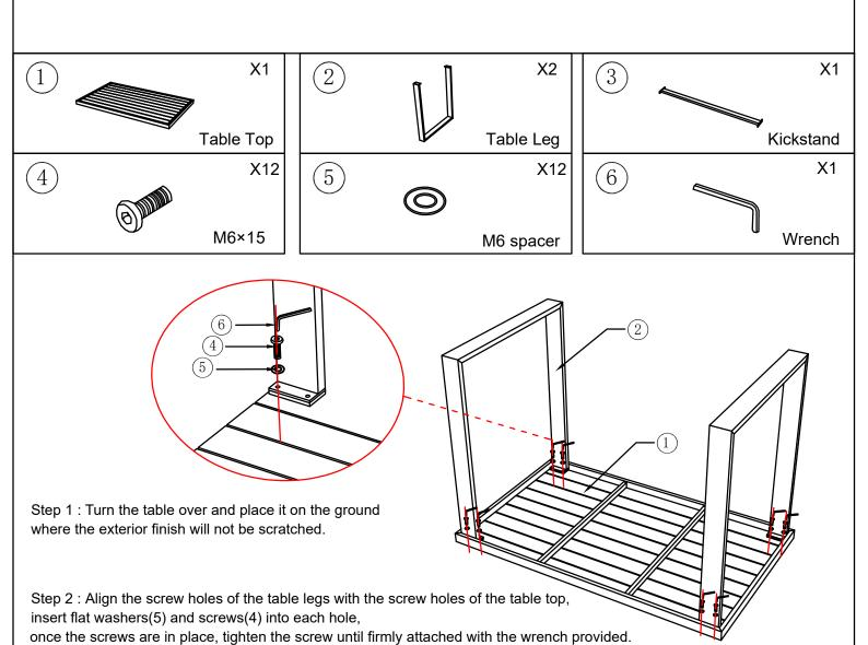
Step 3: Insert the flat washer (5) and screw (4) into each hole, and then install the Kickstand.
