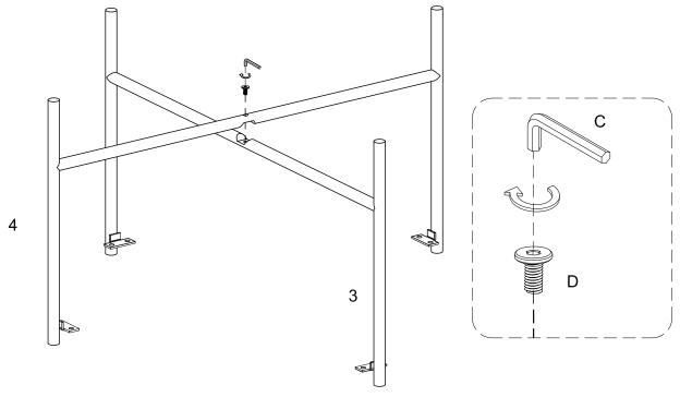
Attach part (4) to part (3) using bolt (D) with hex key (C).
