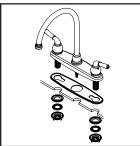
(2) Apply adequate plumbers putty along the boundary of base gasket. Align faucet with mounting holes and place faucet on the sink. Slide washers on shanks and secure the locknuts to the shanks from underneath the sink. Go to step (5) if faucet is without side
