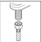
(5) When using stainless steel braided faucet supply hose; this faucet requires one end of the supply hose to have a 1/2" female IPS connection. The other end of this supply hose must match the thread on the water supply valve under your sink. Once you've identified the required size, carefully follow the manufacturer's installation instructions for
