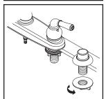
(3) Place side spray holder on mounting hole. Tighten locknut from underneath the sink to secure side spray holder.
