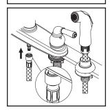
(4) Lead side spray hose through side spray holder. Insert spray head hose quick connect adapter into faucet outlet hose end, push until a "click' is heard. Pull side spray hose downward to test engagement.
