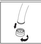
(6) Important: After installation is complete, remove the aerator. Turn on the water and allow both hot and cold water to run for at least one minute each. While water is running, check for leaks. Turn off the water and replace the aerator when finished.
