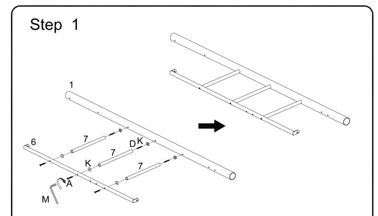
Attach post (1) to the left side of ladder rungs (7) using double-ended screws (D) and rounded washers (K). Attach ladder rail (6) to the right side of ladder rungs (7) using medium bolts (A) and rounded washers (K). Tighten medium bolts (A) with small wrench (M).
