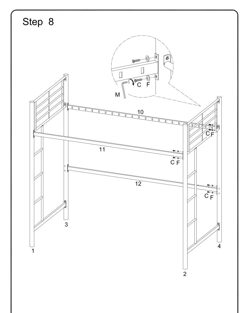
Attach crossbars (10,11,12) to the assembly from Step 6 using small bolts (C) and small washers (F). Tighten small bolts (C) with small wrench (M).
