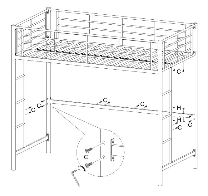
Screw small bolts (C) and insert plastic plugs (H) into the bunk bed assembly. This will fill the holes that are used only with the optional accessory attachments, which are sold separately.
