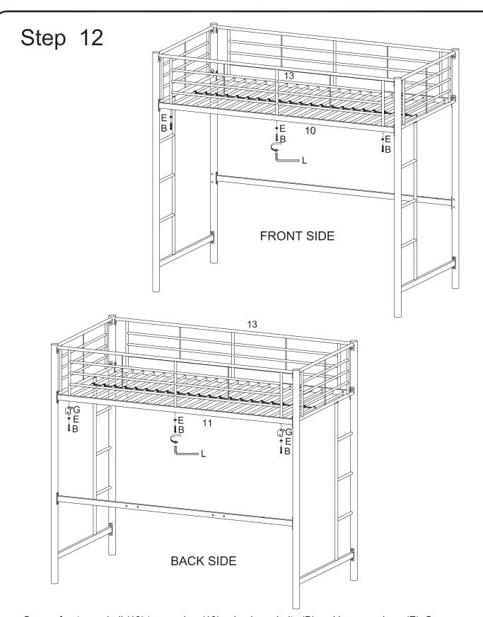
Secure front guardrail (13) to crossbar (10) using large bolts (B) and large washers (E). Secure back guardrail (13) to crossbar (11) using large bolts (B), large washers (E) and, where applicable, angle brackets (G).\* Tighten large bolts (B) with large wrench (L).
