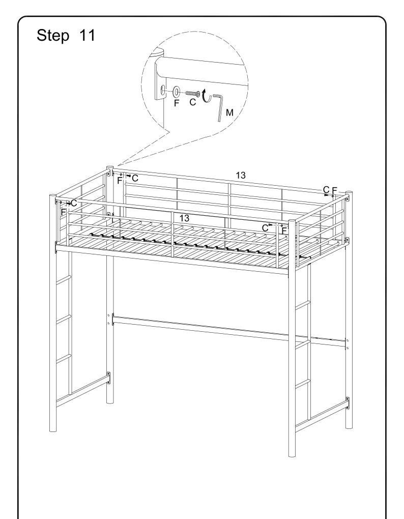
Attach guardrails (13) to posts (1,2,3,4) using small bolts (C) and small washers (F). Tighten small bolts (C) with small wrench (M).
