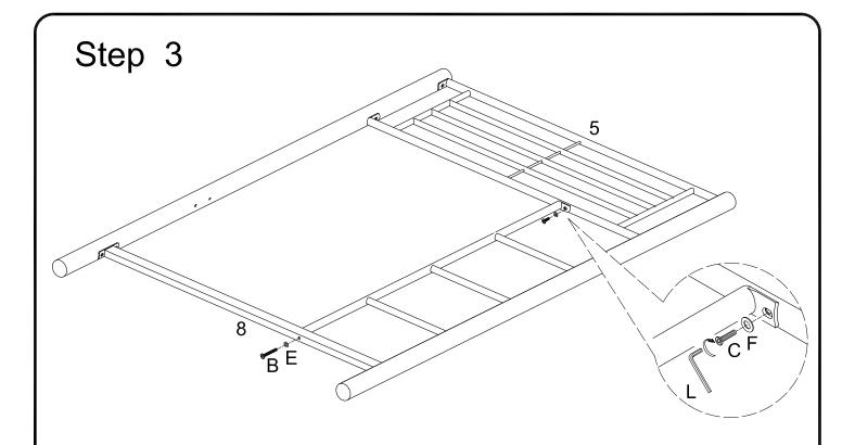
Secure ladder rail (6) to guardrail (5) using small bolt (C) and small washer (F). Secure ladder rail (6) to crossbar (8) using large bolt (B) and large washer (E). Tighten small washer (F) with small wrench (M) and large bolt (B) with large wrench (L).
