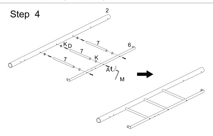
Attach post (2) to the right side of ladder rungs (7) using double-ended screws (D) and rounded washers (K). Attach ladder rail (6) to the left side of ladder rungs (7) using medium bolts (A) and rounded washers (K). Tighten medium bolts (A) with small wrench (M).
