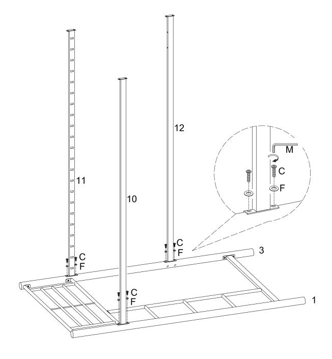
Attach crossbars (10,11,12) to the assembly from Step 3 using small bolts (C) and small washers (F). Tighten small bolts (C) with small wrench (M).
