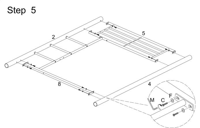
Attach guardrail (5) and crossbar (8) to post (2) using small bolts (C) and small washers (F). Attach post (4) to guardrail (5) and crossbar (8) using small bolts (C) and small washers (F). Tighten small bolts (C) with small wrench (M).
