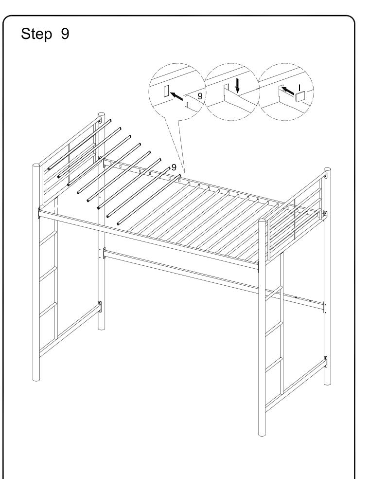
Insert mattress support bars (9) into the provided slots of crossbars (10,11). Secure mattress support bars (9) by snapping plastic tab locks (I) into the provided slots of crossbars (10,11). Note that it may be necessary to apply more pressure to some plastic tab locks than others.
