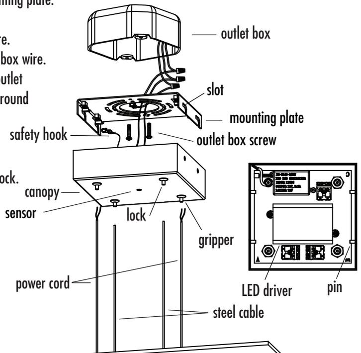
**NOTE: This fixture is controlled by the included IR remote control, which must be aimed at the sensor in the center of the canopy. The fixture may be turned on/off by a wall switch, but do not use with a wall dimmer, or damage will occur.**
