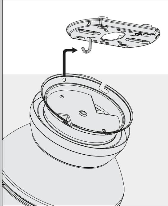
**DO NOT PICK THE FAN UP BY THE WIRES.** Use the hanging hole on the body of the fan to hang the fan on the hook of the ceiling mounting plate.
