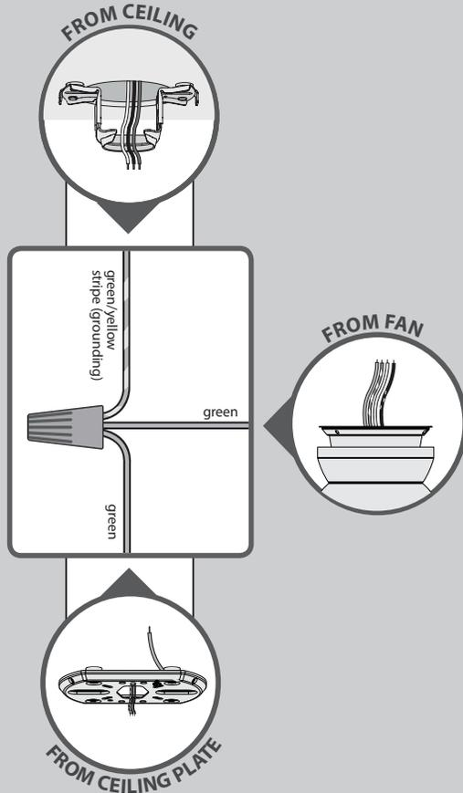
Using an orange wire connector:
