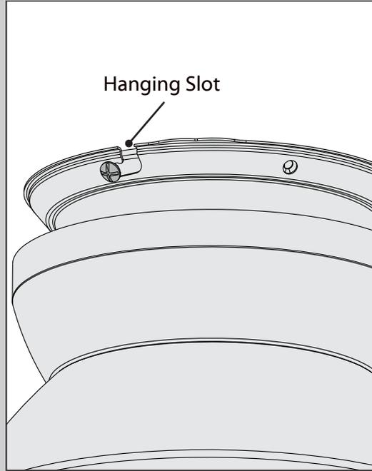
Using both hands, lift the fan body from the hook and align the hanging slots on both sides of the fan body with the two partially installed canopy screws. Slide the two slots on both sides of the fan body between the head of the screws and rotate the fan body clockwise so the screws hold the fan body firmly in place.
