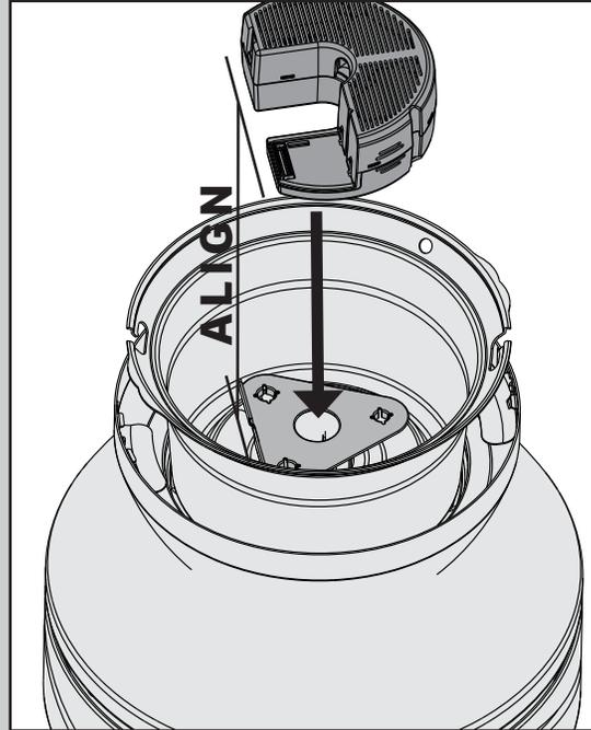
Align the flat side of the control receiver with the flat side of the triangular seat. Lower the control receiver on the triangular seat. Ensure the posts on the bottom of the control receiver are seated in the holes in the triangular seat.
