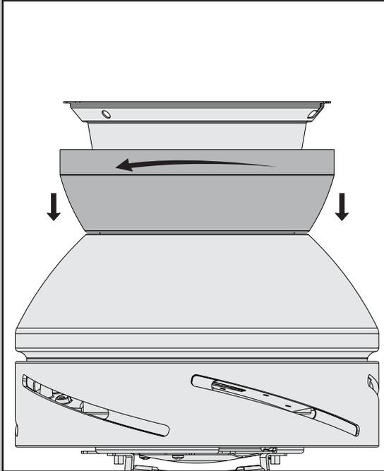
Unlock the canopy cover from the canopy ring tabs to loosen the canopy ring and lower it down to the fan body as shown.
