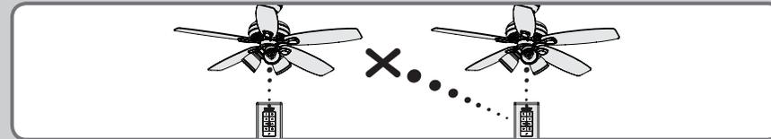
If a transmitter is mistakenly operating a fan, you need to “unpair” the transmitter from that fan’s receiver. The “unpairing” procedure is the same as the pairing procedure.
