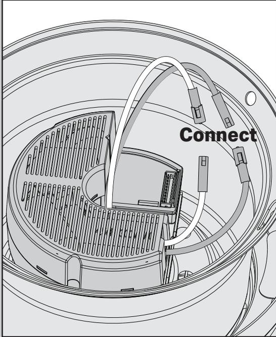
Locate the single-pin connectors that are taped together. Connect the single-pin connectors from the control receiver to the connectors from the fan. Connect the white wires together. Connect the blue wires together. The third, loose wire will not be used for your installation. It is capped to prevent usage.
