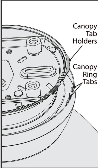
Before going to the next step, locate the two sets of canopy ring tabs that are on the top edge of the canopy and the two sets of canopy tab holders found at the top of the fan body near the ceiling.
