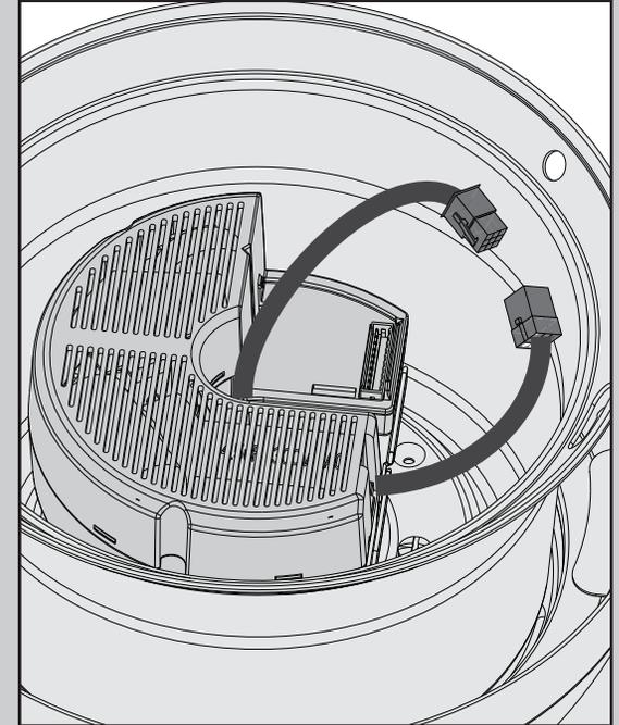
Connect the larger plug connectors together. Make sure to line up the colored markings on the connectors. Ensure that the plugs latch together.
