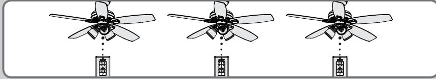
To install multiple fans with independently operating remote controls, **there is no need to perform any pairing procedures**. Each set of receiver/transmitter is already paired. Simply install each receiver into a fan and use the appropriate transmitter to operate each fan.
