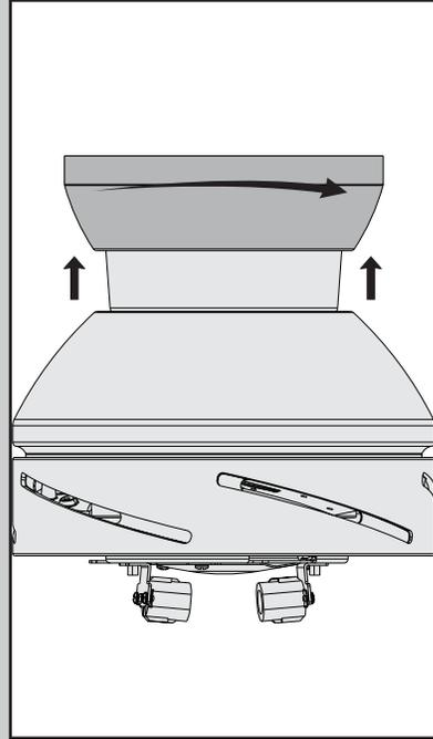
To install the canopy ring, lift the canopy, then rotate clockwise until the tabs are held in place by the tab holders, locking the canopy ring into place.
