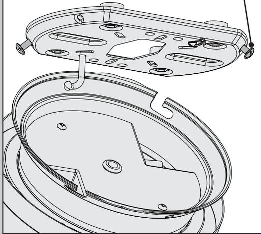
Partially install two of the canopy screws into screw holes on opposite corners of the ceiling plate as shown. Choose the two screw holes that are aligned with the hanging slots in the fan body.
