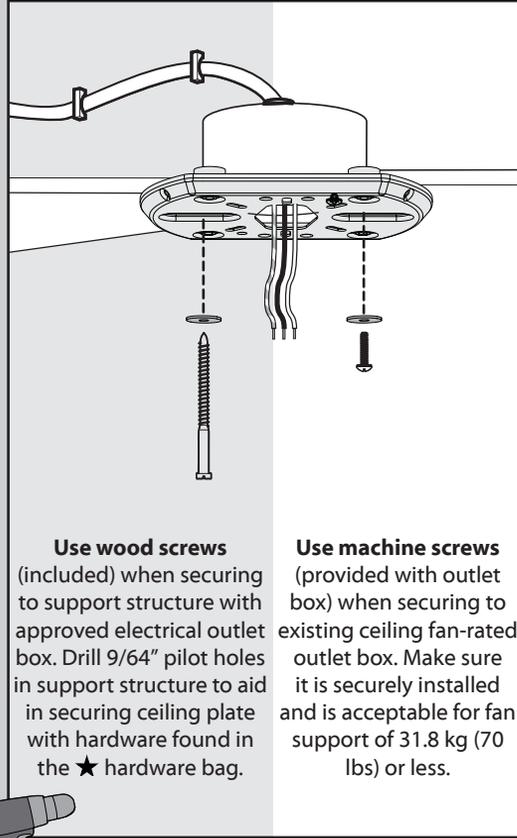
**Use wood screws** (included) when securing to support structure with approved electrical outlet box. Drill 9/64" pilot holes in support structure to aid in securing ceiling plate with hardware found in the ★ hardware bag.
