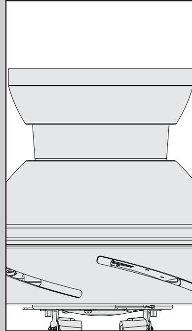
To check your work, make sure there is an even gap all the way around between the ceiling and the canopy ring.
