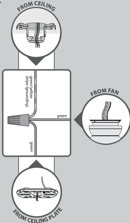
Using an orange wire connector:
