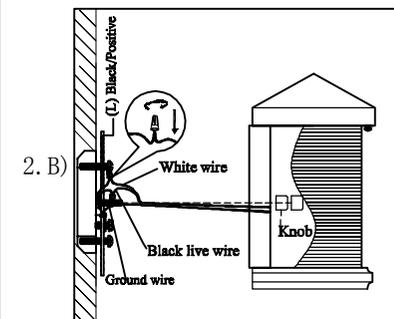
Step.2 Wire fixture to wires in outlet box. Black wire is positive, white is neutral, bare wire is ground.
