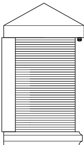
To prevent water intrusion, caulk around post cup where fixture meets the wall using outdoor silicone sealant.
