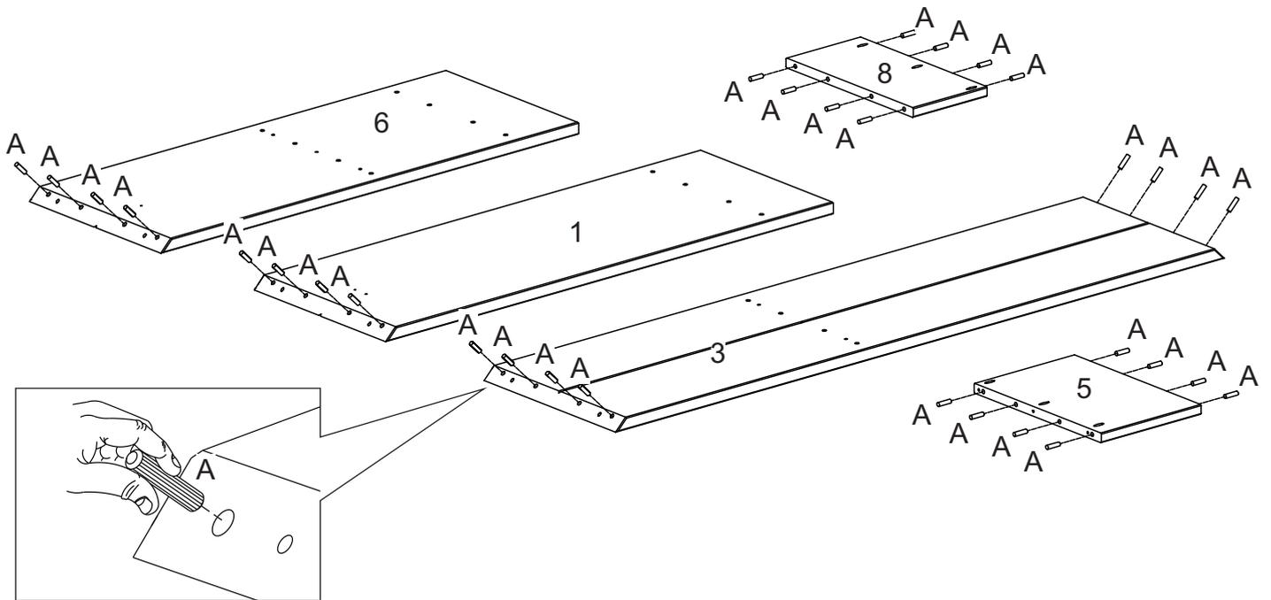
Insert Wooden dowel (A) into part (1), (3), (5), (6) and (8).
