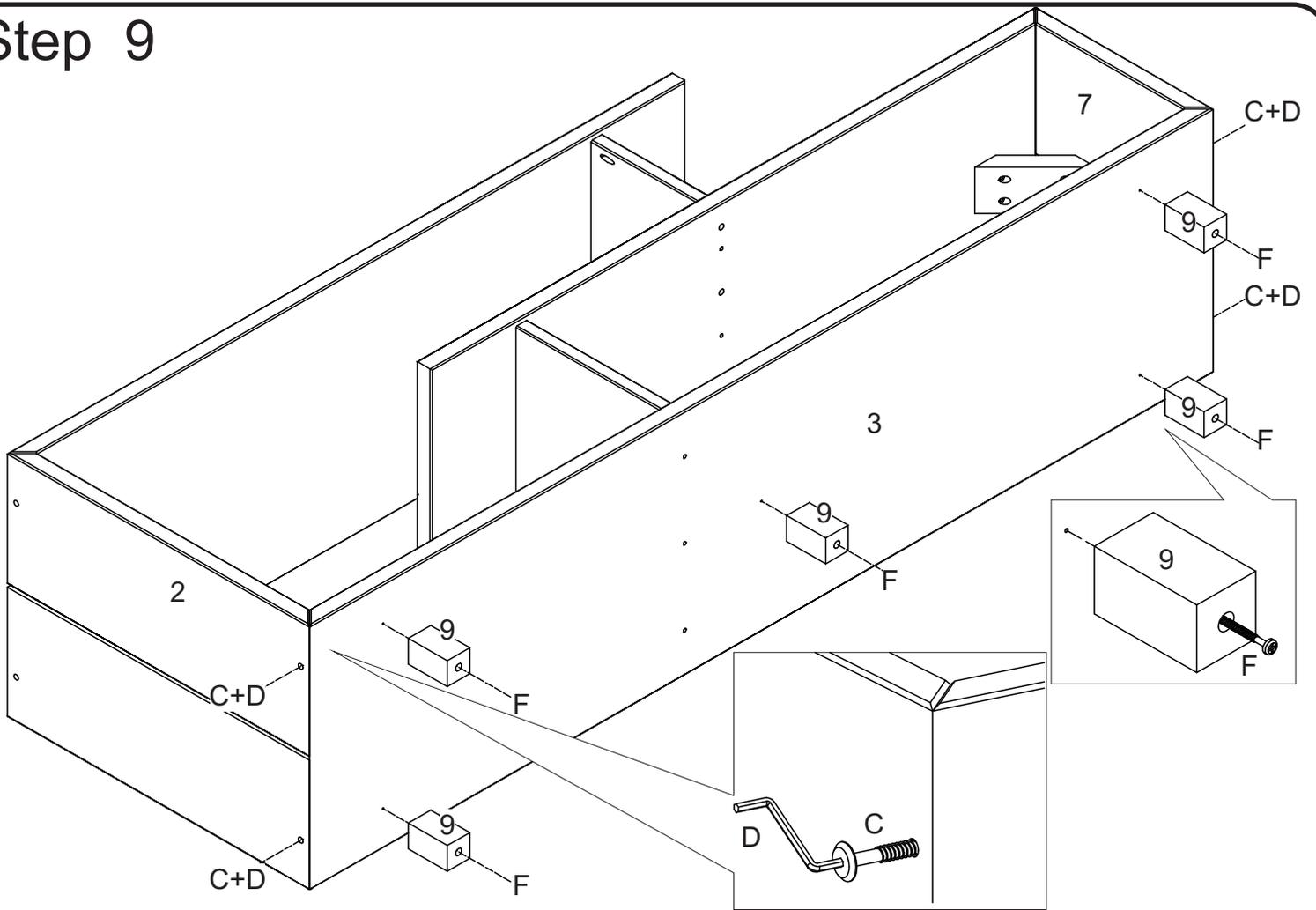
Secure part (3) to part (2), (7) with screw (C) and hex key (D). Secure part (9) to part (3) with screw (F).
