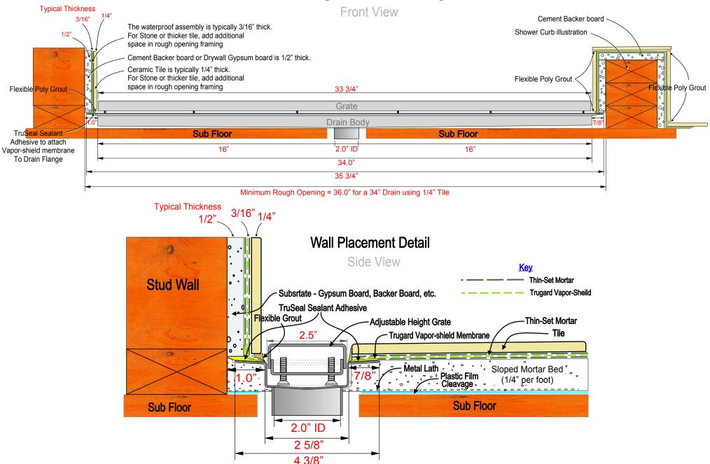
Note: To determine the framing rough opening size, add one inch to the length or width of the drain body, if a one quarter inch thick tile is being used. If the tile or stone is thicker than the 1/4" and the additional thickness of the tile to the 1 inch distance normally used to determine the rough opening size. So for example, for the rough opening for a 34 inch linear drain, the rough opening would need to be 36 inches, when 1/4" tile is being used.
