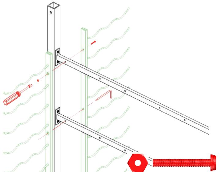
**3. Assemble presentation rack** – Position presentation racks back to back as shown. Using nut driver (included), a Phillips head screwdriver (not included) attach presentation racks with presentation rack assembly screws. Fully tighten.
