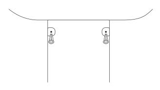
3. Slide shroud into place and secure using same steps as when mounting the sink. Use cover caps to hide hardware. Do not overtighten, it may crack the ceramic.
