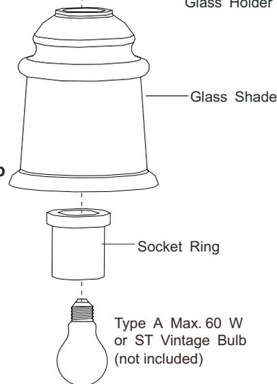
5. Attach the glass shades onto the glass holders and tighten them with the socket rings.
