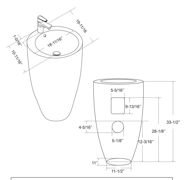
**ATTENTION!** Dimensions may vary by up to 3/8". It is highly recommended to pull all dimensions of actual model for installation and measuring purposes.
