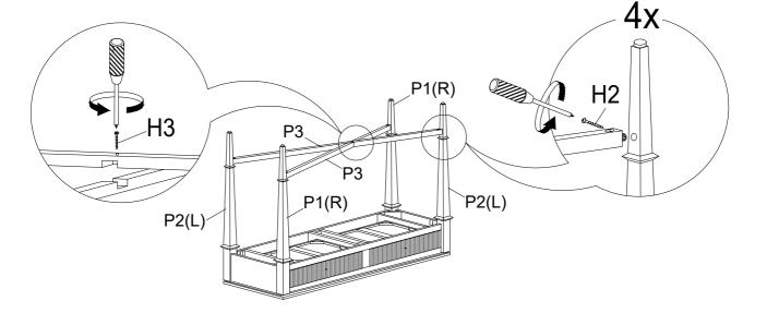
Step 4: Turn the assembled table to an upright position, remove the handle from inner drawer, and attach it on outside of the drawer with screw driver. Assembly is complete.
