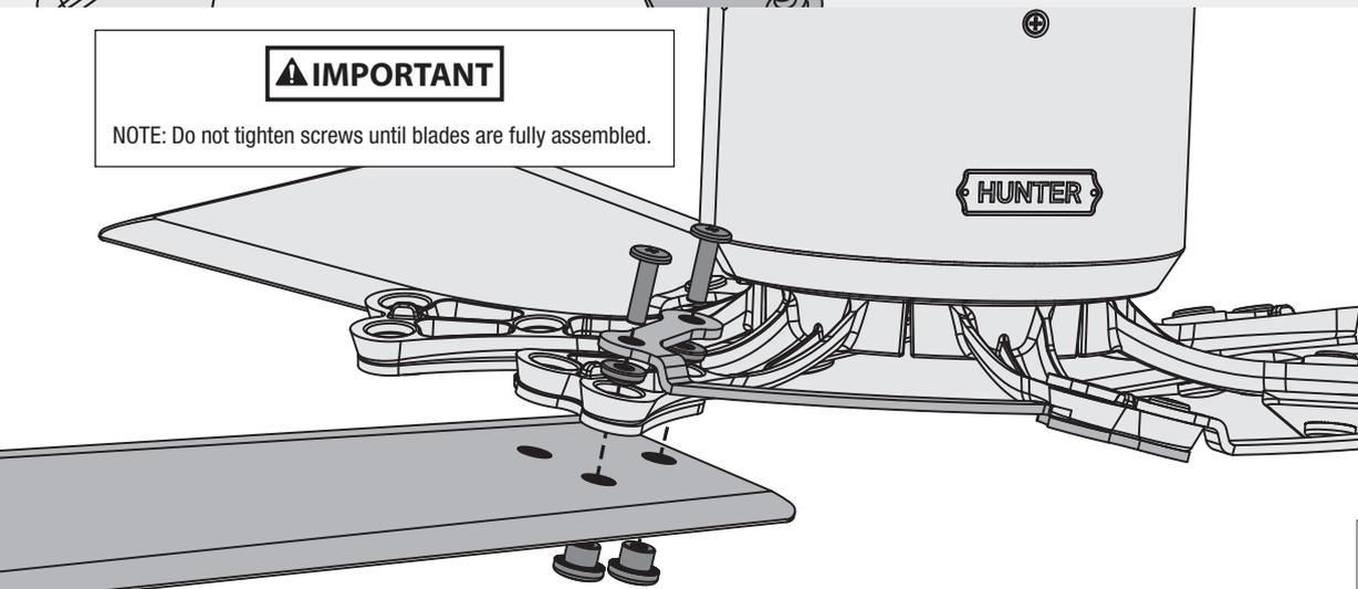
Lightly attach each blade to a blade arm and blade arm connector as shown using the blade nuts and grommets, found in the hardware bag, and the blade assembly screws, found in the bag. Leave the trailing edge hole in the blade assembly open for the following step.
