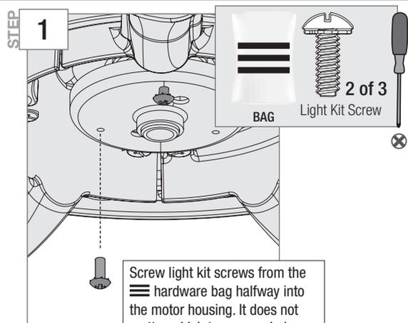
Screw light kit screws from the
