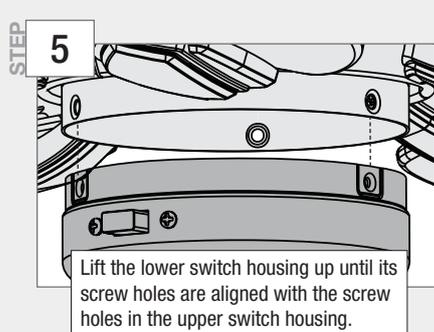
Lift the lower switch housing up until its screw holes are aligned with the screw holes in the upper switch housing.
