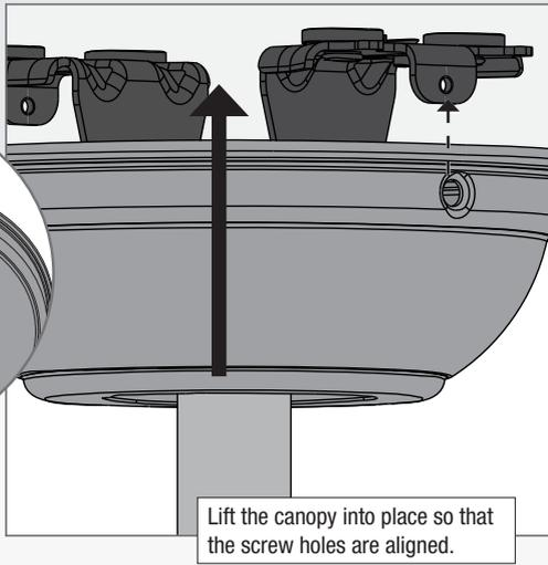
Lift the canopy into place so that the screw holes are aligned.
