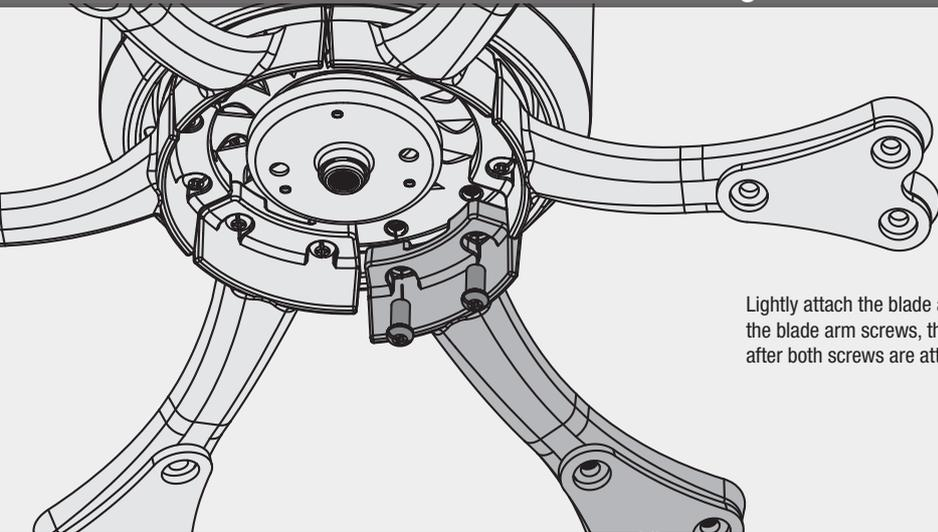
Lightly attach the blade arms to the motor with the blade arm screws, then securely tighten after both screws are attached.
