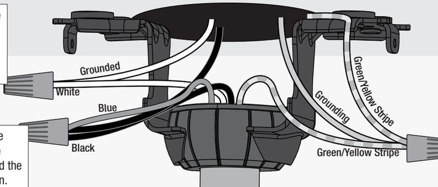
Connect the three grounding wires (green, green/yellow stripe, or bare copper) coming from the ceiling, downrod, and hanging bracket.
