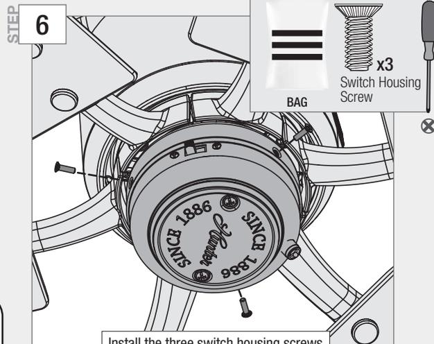
Install the three switch housing screws found in the
