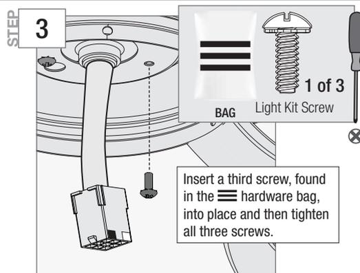
Insert a third screw, found in the
