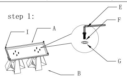
Fit the adjust legs (I) to bottom base, Connect Stainless steel pillar (B) with Stainless steel base (A) by Screw (F) (M8\*20), tighter, one by one
