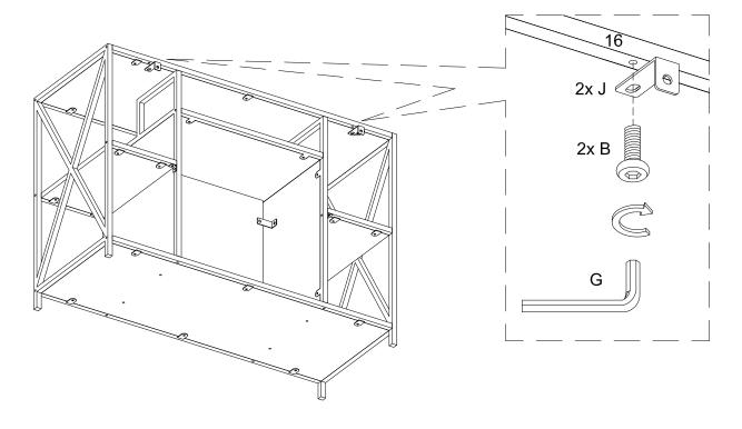
Attach bracket (J) to back frame part (16) using bolt (B) with hex key (G).
