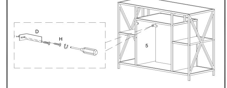
Secure the fireplace (15) to the frame part (5) using bracket (D) and screw (H).
