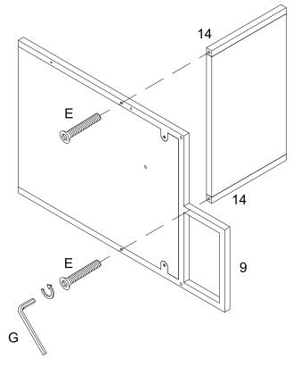
Attach part (14) to part (9) using bolt (E) and Hex Key (G).
