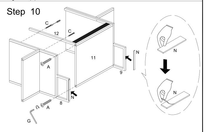
Attach part (8) to part (11, 12) with bolt (A) and Hex Key (G). Attach part (12) to part (8) using screw (C) and a screwdriver. Place Foam Pad (N) on part (8, 9) as per diagram.
