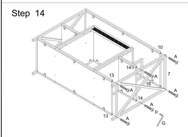
Attach part (7) to part (10,13,14,16) using bolt (A) and Hex Key (G).
