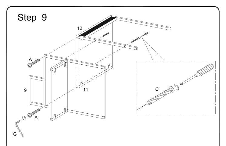
Attach part (9) to part (11,12) using bolt (A) and Hex Key (G). Attach part (12) to part (9) using screw (C) and a screwdriver.
