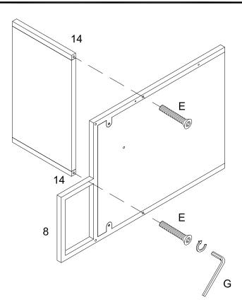
Attach part (14) to part (8) using bolt (E) and Hex Key (G).
