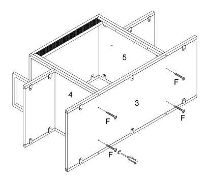
Secure part (3) to part (4,5) using screw (F) and a screwdriver.
