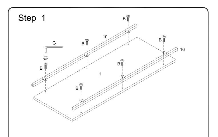
Attach part (10,16) to part (1) using bolt (B) and Hex Key (G).
