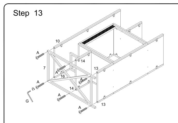
Attach part (7) to part (10,13,14,16) using bolt (A) and Hex Key (G).
