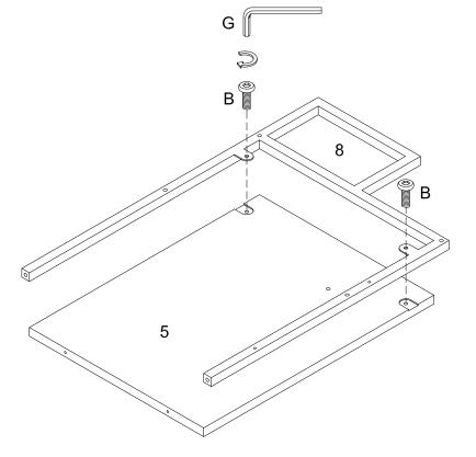
Attach part (8) to part (5) using bolt (B) and Hex Key (G).
