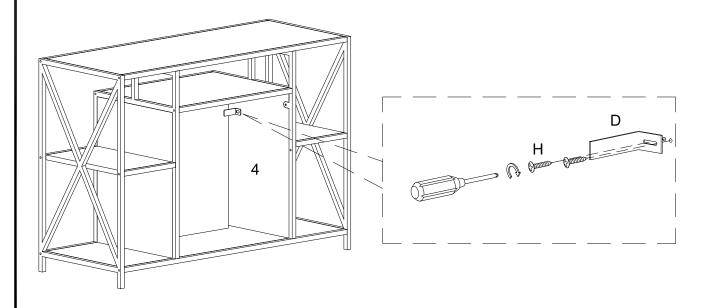
Secure the fireplace (15) to the frame part (4) using bracket (D) and screw (H).
