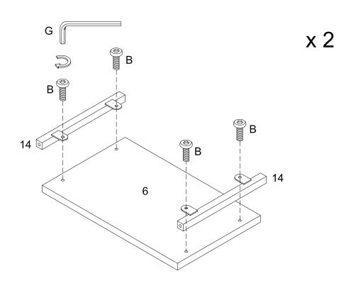
Attach part (14) to part (6) using bolt (B) and Hex Key (G). Complete this step twice.
