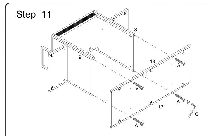
Attach part (13) to part (8,9) using bolt (A) and Hex Key (G).
