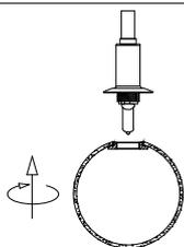
Attach the glass to the holder, and rotate in a clockwise direction gently.
