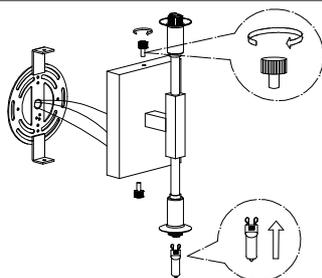
Attach the fixture to the mounting plate with screws provided.
