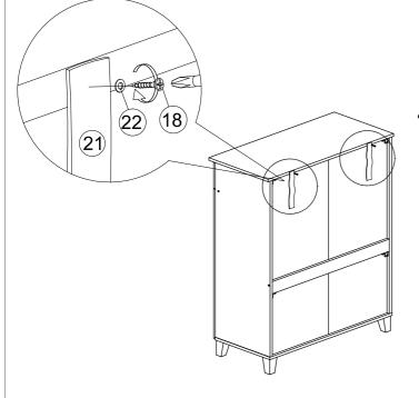
4. Add safety strap (21), washer (22) using 3.5x15mm screw (18) to back of cabinet.
