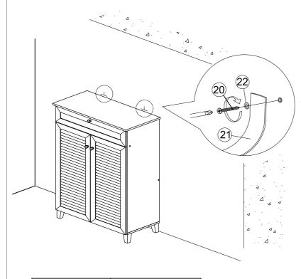
5. Finally, attach safety strap (21) and washer (22) using 4x30mm screw (20) to the wall.
