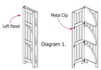
1. Open the left panel and right side panel of corner shelf as shown in Diagram  $1. \,$
