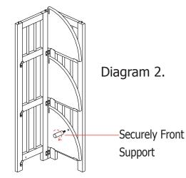
2. Put the front support (MS0952V) into the hole under the Bottom shelf as per Diagram 2.
