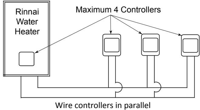
The 4 temperature controllers can consist of multiple MC-91-2 or MCC-91-2 but only one BC-100V and only one MC-100V.
