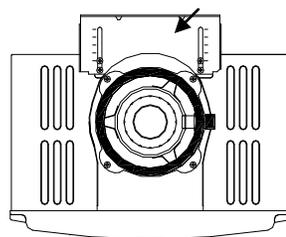
To adjust the condensate collector position or to replace the female vent top with a male vent top:
