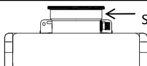
Secure the first vent component to the water heater with one self-tapping screw at the hole located above the condensate collector.
