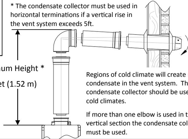
Regions of cold climate will create more condensate in the vent system. The condensate collector should be used in cold climates.
