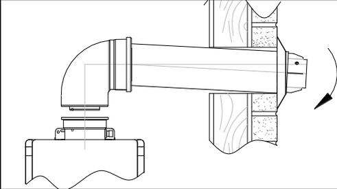
\* The condensate collector must be used in horizontal terminations if a vertical rise in the vent system exceeds 5ft.
