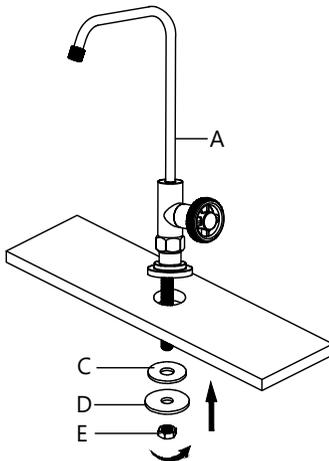
Place the faucet assembly (A) through the selected hole in the sink or countertop. On the underside of the sink or countertop, slide the rubber washer (C) and metal washer (D) onto the stud. Thread the mounting nut (E) onto the stud, and tighten securely using your wrench.
