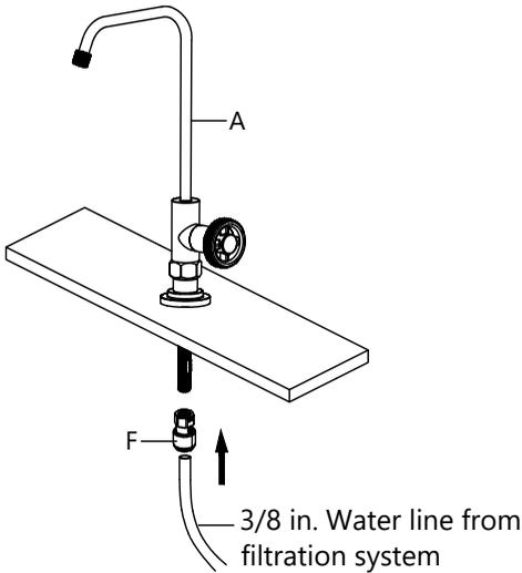
Thread the quick connect adaptor (F) onto the end of the faucet assembly (A) stud, and tighten securely using a wrench. Connect the 3/8 in. water line from the filtration system by pushing the line into the connector (F). Pull down on the 3/8 in. line slightly to ensure the quick connect fitting has engaged.
