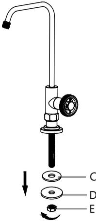
Remove the rubber washer (C), metal washer (D), and mounting nut (E) from the end of the stud.
