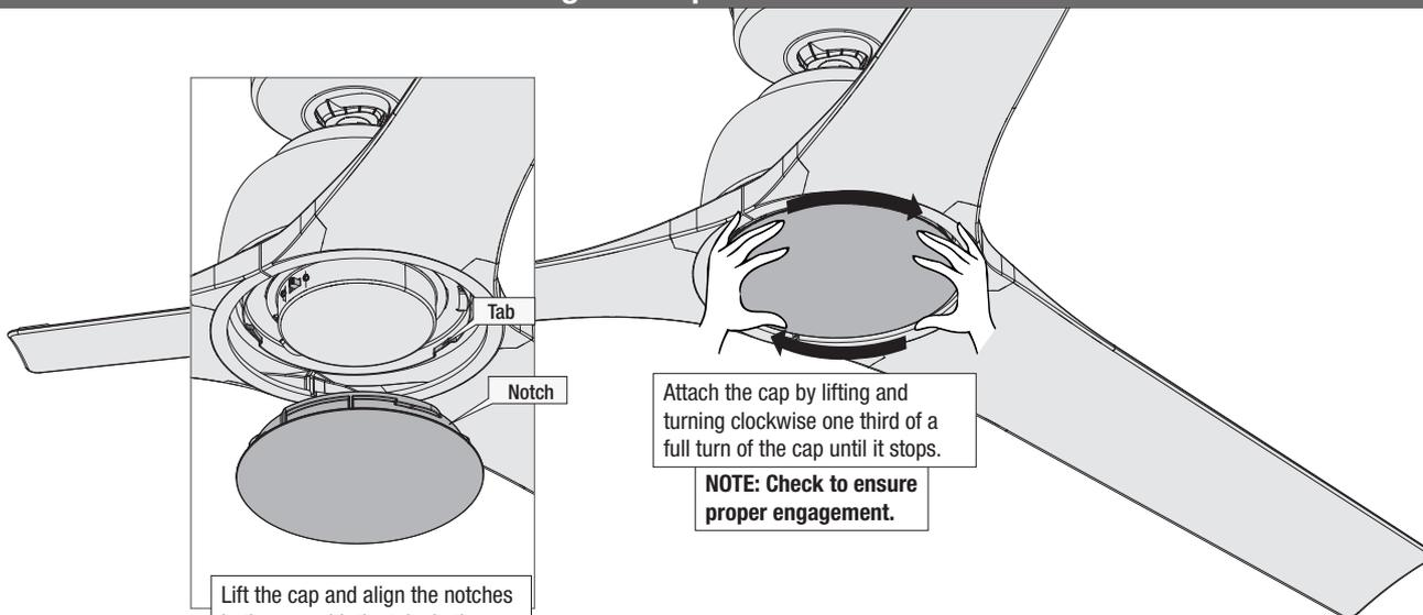
Lift the cap and align the notches in the cap with the tabs in the upper switch housing.
