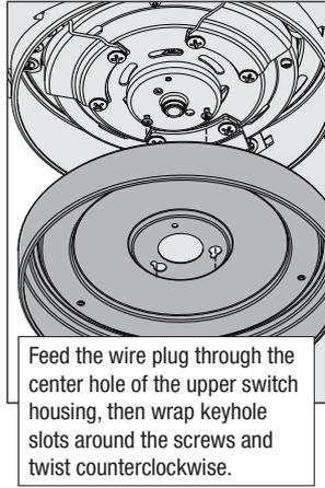
Feed the wire plug through the center hole of the upper switch housing, then wrap keyhole slots around the screws and twist counterclockwise.
