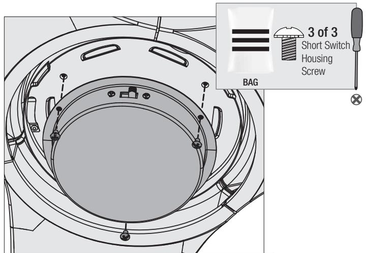
Lift the lower switch housing until its screw holes are aligned with the screw holes in the upper switch housing. Install the three short switch housing screws, found in the hardware bag. Tighten all three screws.
