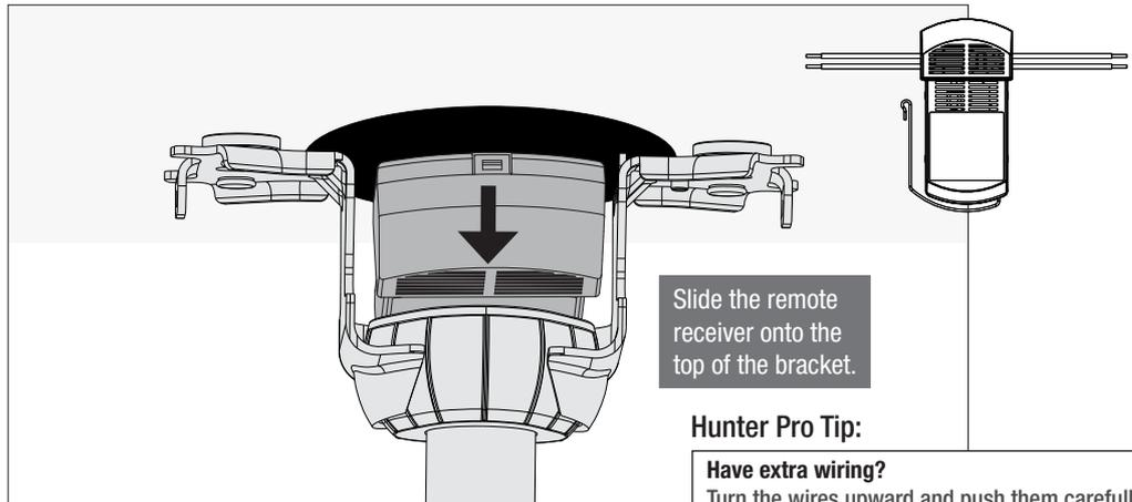
Slide the remote receiver onto the top of the bracket.
