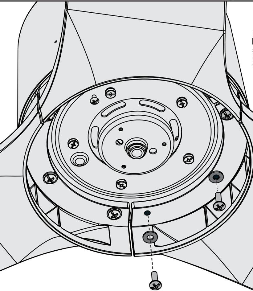
Put the blade washers found in the ■ hardware bag onto the blade screws found in the ▲ hardware bag. Then install the blade screws to secure each blade to the fan.
