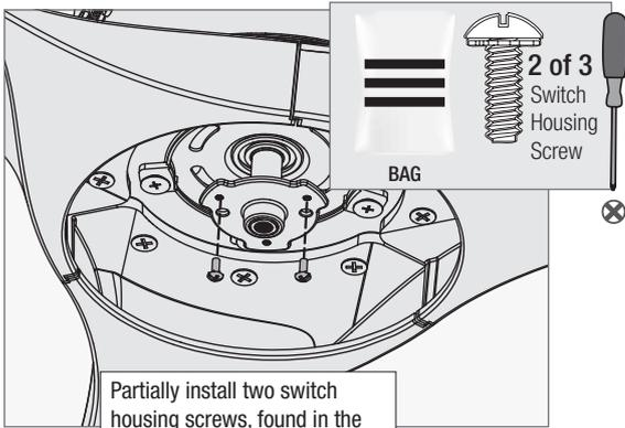
Partially install two switch housing screws, found in the hardware bag, halfway into the motor housing as shown. It does not matter which two screw holes you choose.
