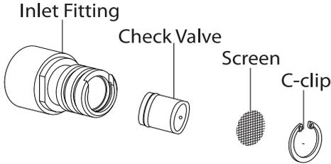
Remove C-Clip, Screen, and Check Valve. Rinse with water to clean debris. Reinstall in Inlet Fitting.
