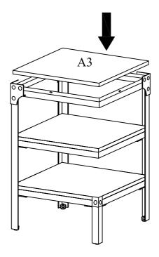
Place Top Panel A3 onto Top Frame A2 as shown above.
