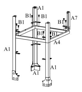
Assemble Bottom Shelf Frame A4 to Legs A1 and Leg A7 using Bolts B1. NOTE: Please do not tighten Bolts B1 until Step 7.
