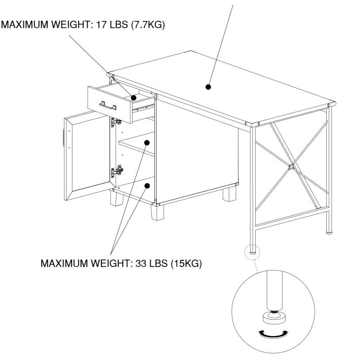
Use the provided screw, to adjust the balance of the cabinet by attaching it to the bottom of the leg.
