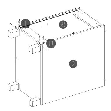
Peel off the adhesive sticker's protective paper and bond it onto the designated position before secure with nails.
