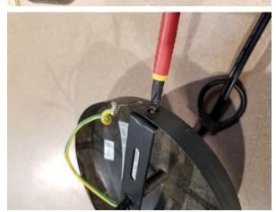
Remove 2 Screws On Sides and slide cap down the wire. Be sure you keep the wire going through the cap Hole before you proceed to next step.
