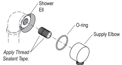
**NOTE:** A hex wrench can be used to tighten the threaded adapter.
