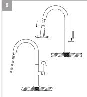
Unscrew spray head by hand. Hold the tip of the spray hose down and turn on the faucet and let the water run 60 seconds to flush any debris, the re-connect spray head. Ensure gasket is present.
