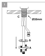
Ensure there is a Ø35mm through-hole on the kitchen counter. Remove the mounting nut (A) and washer (B) from the threaded shroud (C).
