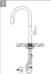
Connect pullout hose to quick connect and insert weight (loose-install).
