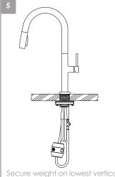
Secure weight on lowest vertical point on pull-out hose side. (not on quick connect side)
