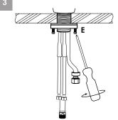
Position faucet on the installation surface. Fit flexible hoses through hole on countertop or sink.
