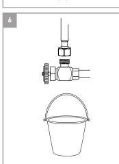
Before connecting supply hose, flush supply valves to clear any debris. Place a bucket underneath valves and run water for 5 to 10 seconds. Turn water off.
