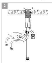
Connect braided supply hoses to faucet female outlets, secure firmly by hand until hose is snug to pipe.
