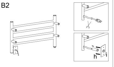
All electrical connections in the junction box must be performed by a fully qualified electrician.
