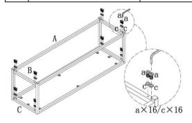
Step 1:Assemble the iron leg firstly as shown picture.
