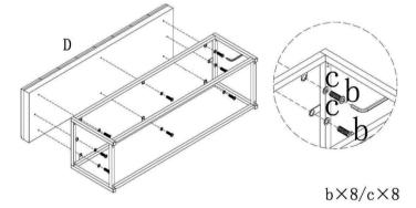
Step 2:After iron leg ready,attached the leg to bench top by screw and round washer with allen wrench.
