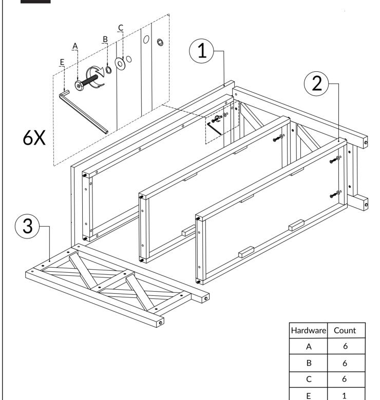
TIGHTEN BOLT COMPLETELY.
