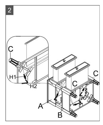
Step 2. Attach 2 legs (C) with top cabinet (A) and bottom cabinet (B). Using Allen key (H2) to lock with 8\*bolts (H1).
