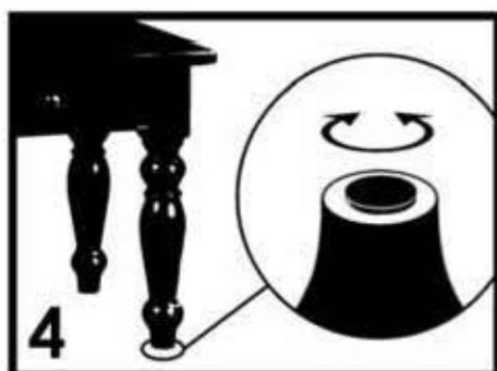
4 Some furniture come with optional **height adjustment knobs** underneath each leg. Turn this knob counterclockwise to raise the leg level or clockwise to lower the leg level.
