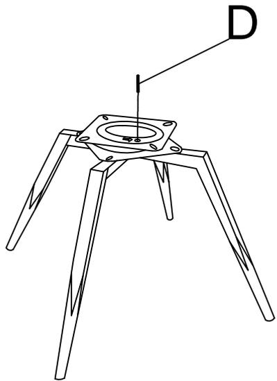
Turn around the rotated plate 45 degree
