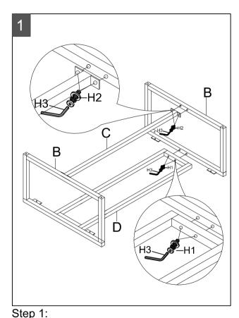
Attach metal top frame (D) to both side frame (B), using Allen Key (H3) to lock with 4\*Allen bolts (H1).
