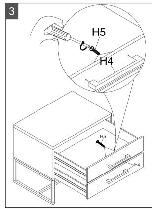
Step 3: Straighten up the assembled night stand, attach 2\*handles (H4) to front of drawer, using Phillips screwdriver (not included) to lock with 4\* Phillips head bolts (H5).
