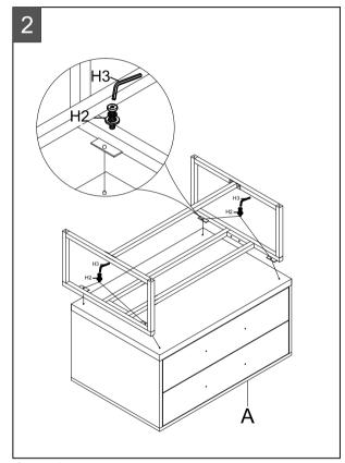
Step 2: Attach the assembled metal base to underneath of cabinet, using Allen Key (H3) to lock with 4\*Allen bolts (H2).
