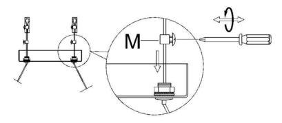
5 » Carefully pass supply wires through mounting plate (A). Secure mounting plate (A) to the outlet box with mounting screws (D).
