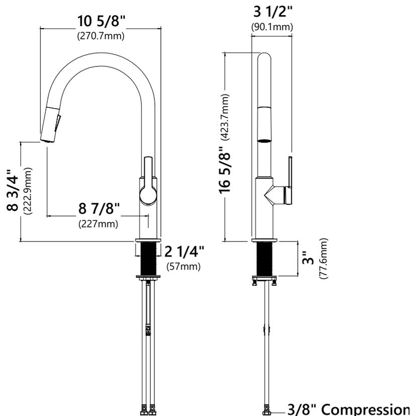
**NOTE:** Some Kitchen Faucets that do not have a pull out or pull down sprayer may be connected to a portable dishwasher. Pull out and pull down faucets should never be connected to portable dishwashers because potential pressure fluctuations during washing cycles cause hose ruptures or leaks.
